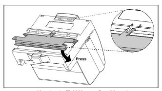
Figure 3. Mounting the FP-3000 onto a Panel Mount Accessory
